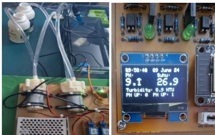
Figure 10. Water pH Sensor Testing Process and Measurement Results Displayed on the OLED Screen
